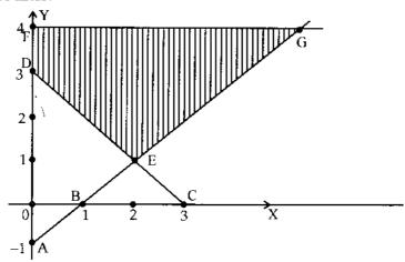
Shaded portion is the feasible region and EDFG is the associated convex polygon. E is the point of intersection of AB and CD. On solving x - y = 1 and x + y = 3 we get E(x, y) = (2, 1). Also F(x, y) = (0, 4)
