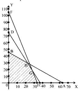
Shaded portion is the feasible region and the associated convex polygon is O E G H B. G is the point of intersection of the lines CD and EF & H is that of the intersection of the lines AB and CD.
