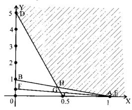
Shaded portion is the feasible region which is unbounded. H is the point of intersection of the line AB and CD. H(x, y) = (4/9, 5/9) obtained by solving x + y = 1, 100x + 10y = 50.
