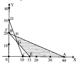
Shaded portion is the feasible region and EAHG is the associated convex polygon. G is the point of intersection of the lines CD and EF. H is the point of intersection of the lines AB and CD.
