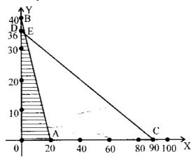
Shaded portion is the feasible region and OAED is the convex polygon. The point E being the point of intersection of lines AB and CD is obtained by solving the equations : 2x + y = 40, 2x + 5y = 180. E(x, y) = (2.5, 35)
