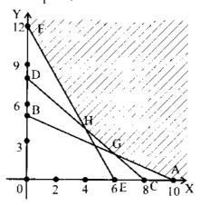
Shaded portion is the feasible region. G is the point of intersection of the lines AB & CD and H is the point of intersection of the lines CD & EF.
