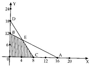
On solving 3X + 4Y = 48 and 9X + 4Y = 72 we get E(X, Y) = (4, 9). The value of the objective function at the vertices of the convex polygon *OCEB* are tabulated.
